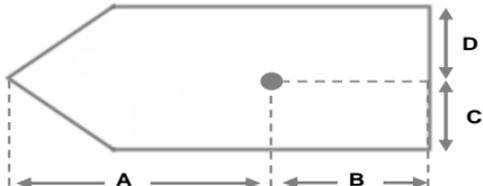
**Figure 3**      **GPS antenna location**
