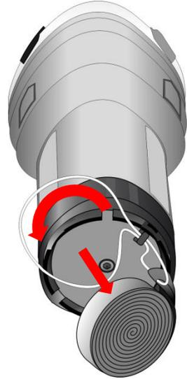
5. Using a 4mm hex key, unscrew retaining bolt until loose. Do not remove at this stage.
