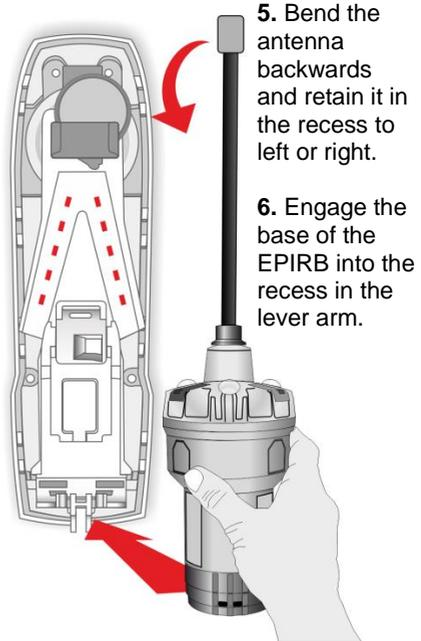
5. Bend the antenna backwards and retain it in the recess to left or right.
