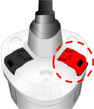
2. Lift the cover, press the ON button for >2 seconds and release.
