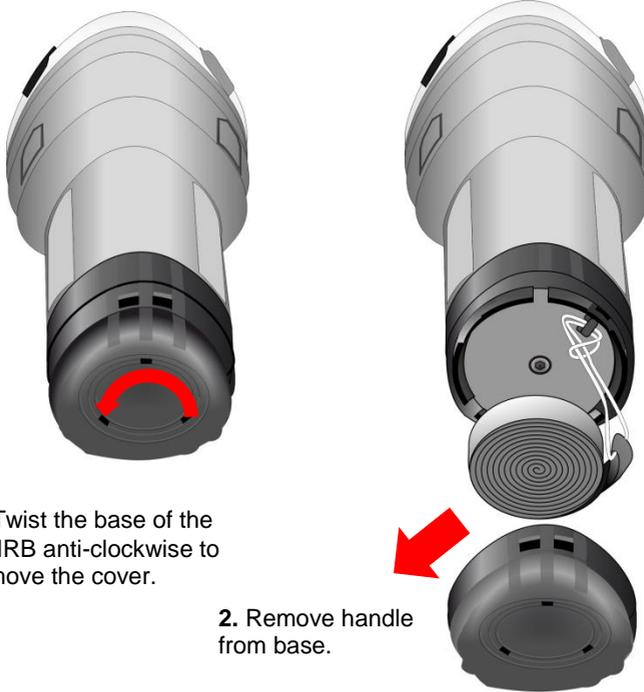
1. Twist the base of the EPIRB anti-clockwise to remove the cover.
