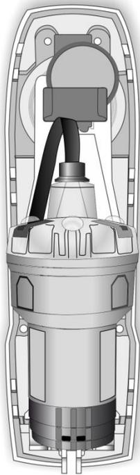
8. Refit cover squarely onto back plate, engaging the guides at the lower end first.
