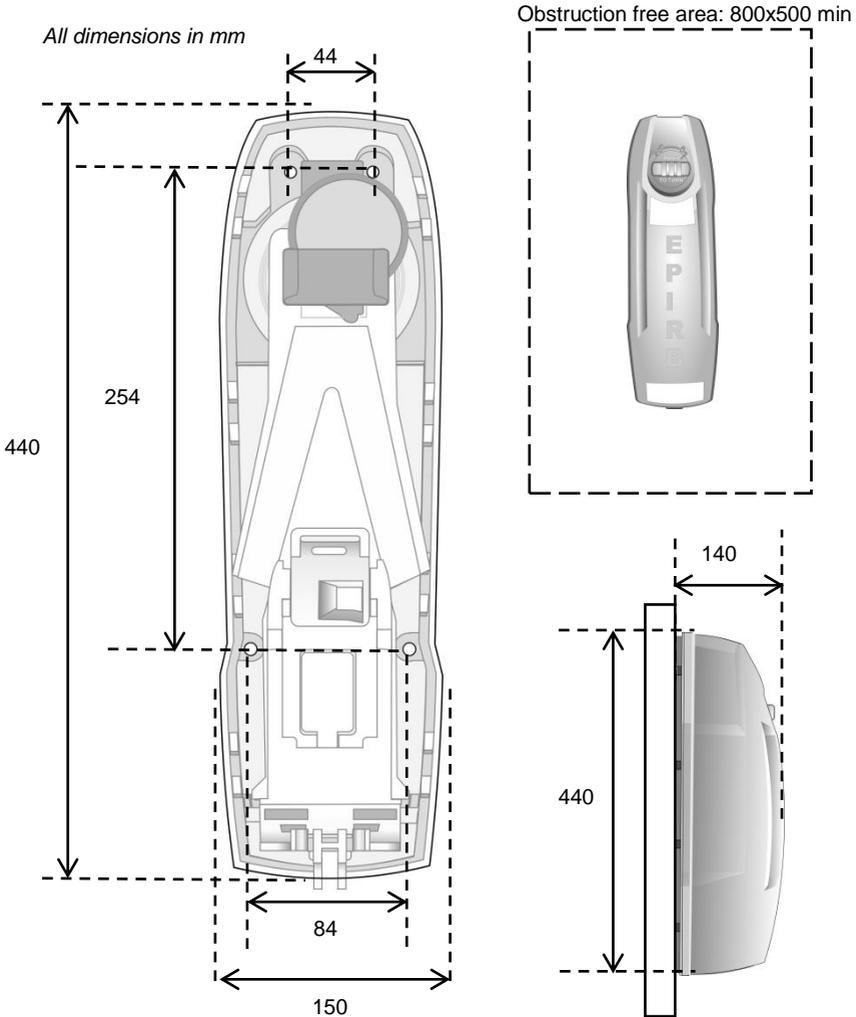
The enclosure is supplied with a set of stainless steel fixings. If the rear of the mounting surface is inaccessible, use self-tapping screws. Offer the back plate into the chosen position and mark through the mounting holes. Drill appropriately sized holes where you have marked. You will need a 4mm hex key to tighten the bolts. Always fit washers under the heads of the bolts to avoid damaging the plastic.
