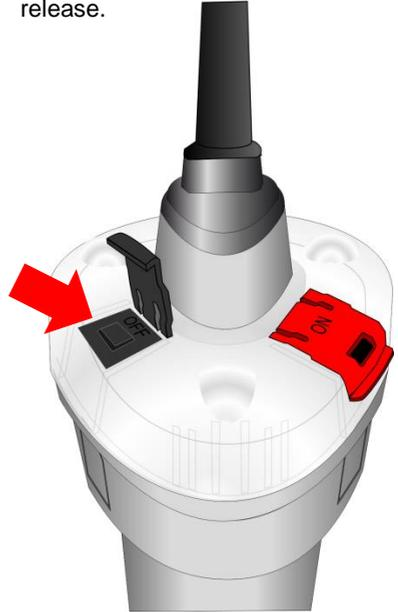
3. The strobe light and green indicator will stop flashing. If any light continues to flash, then check that the sea contacts are dry.
