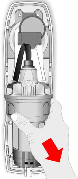
**WARNING – The antenna will spring up when the EPIRB is released. Be careful to avoid eye injury.**
