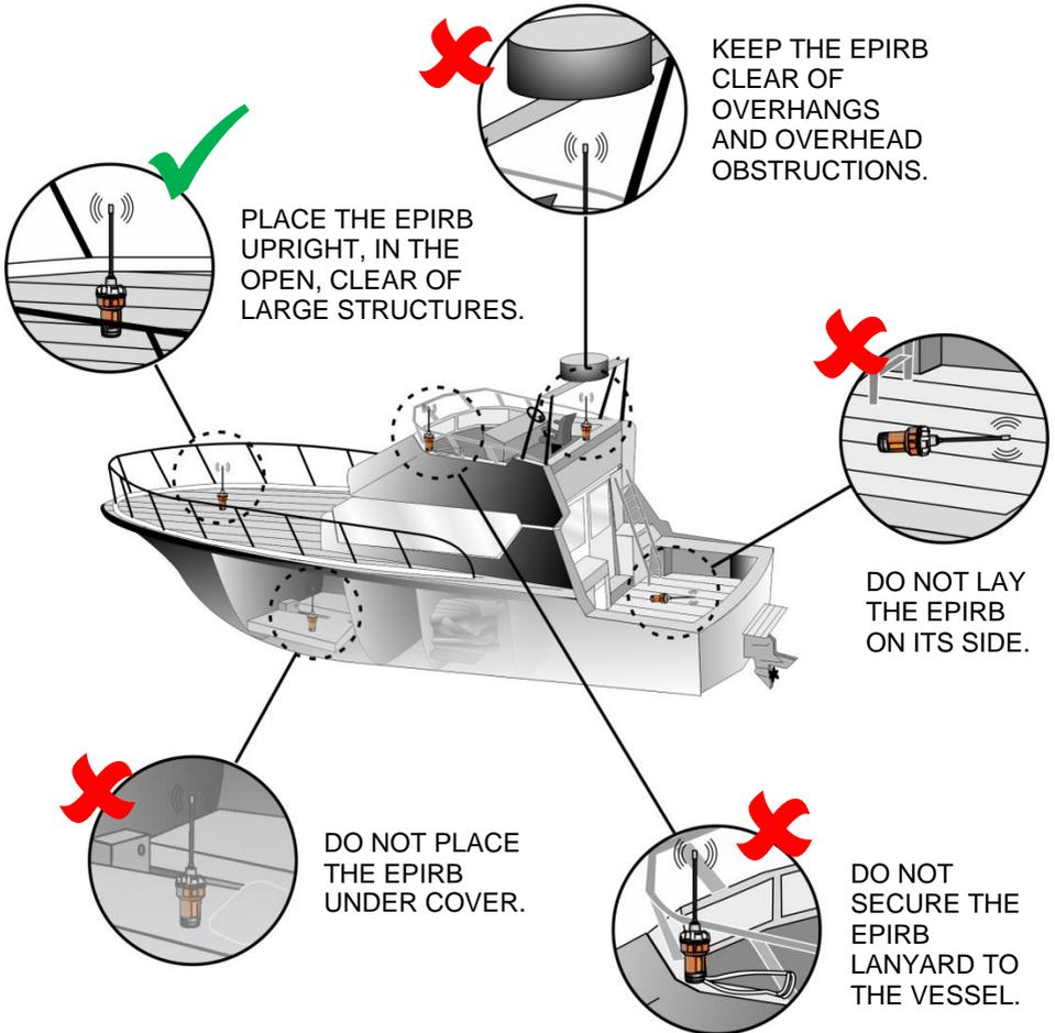
**NOTE:** Failure to observe these guidelines may affect whether and how soon an alert is received by the satellite system. Keep the EPIRB upright at all times (hold it if necessary but do not touch the antenna). The high intensity strobe lights may cause discomfort if viewed for long periods.
