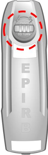
2. Push the dial in and turn anti-clockwise to the unlocked position.
