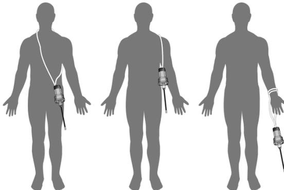
3. Adjust the carry handle to secure the EPIRB across the body, around a shoulder, arm or wrist during emergency evacuation prior to activation.
