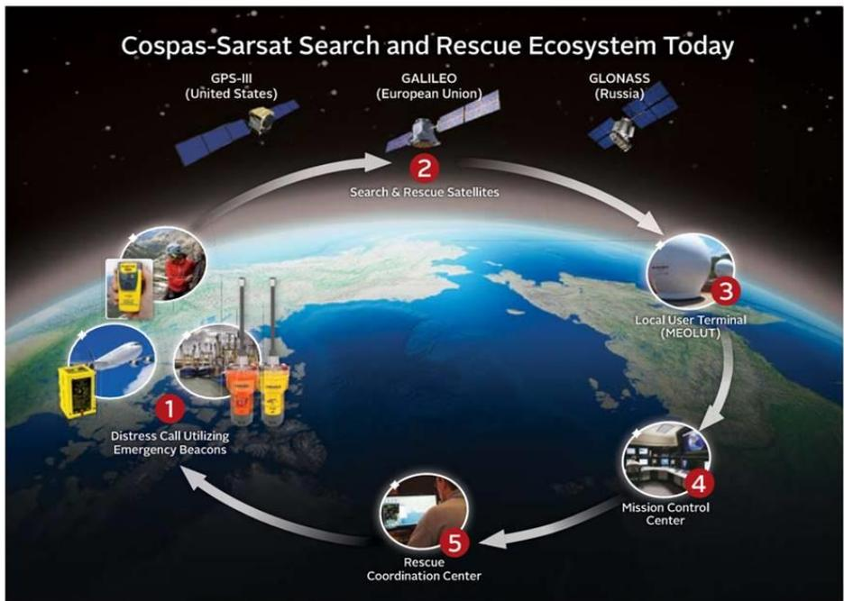
1. The process begins with the activation of a distress beacon (EPIRBs for maritime use, PLBs for personal use and ELTs for aviation use) in an emergency situation, sending out a 406 MHz signal.
