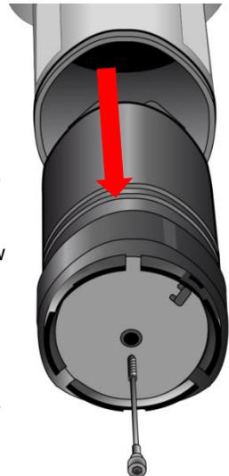
7. Remove the screw completely and dispose of the battery.
