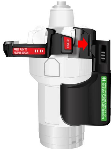
5. Fold over the antenna and locate the tip in the retaining slot behind the EPIRB.
