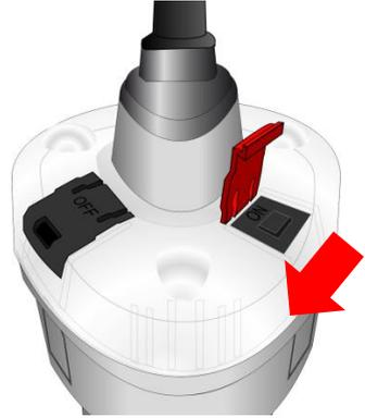
The strobe light will start to flash immediately; however, the EPIRB will not make any distress transmissions for approximately 50 seconds. This allows time to turn off the EPIRB if it has been activated accidentally. When the green indicator starts to flash, distress transmissions have started.
