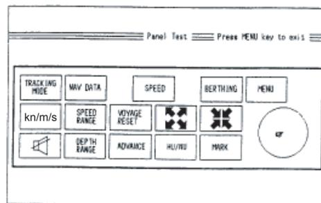
Press each key to see if the corresponding key mark on the screen is highlighted in reverse video. For the trackball, check that the hand pointer (☞) on the screen moves within the circle as the trackball is operated.
