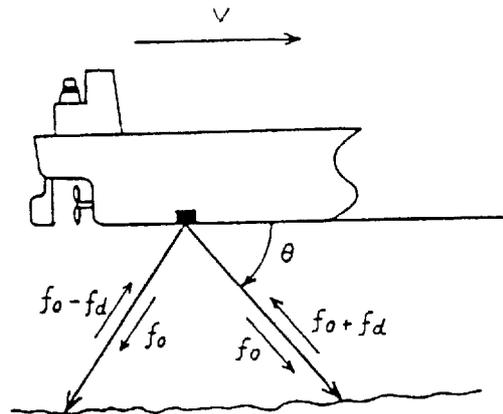
This relative motion causes the Doppler shift and the ultrasonic waves reflected at the seabed are received at frequencies of "fo + fd" and "fo - fd" by the transducer. In the processor unit of the DS-30, difference of "fo + fd" and "fo - fd" are computed to extract only the Doppler shift factor "fd".
