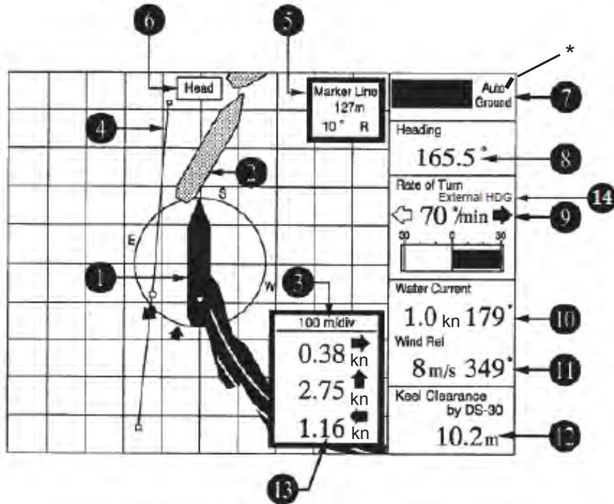
\*: Bar mark rotates at normal condition.
