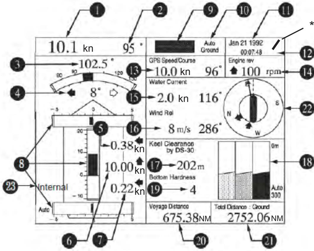
\*: Bar mark rotates at normal condition.
