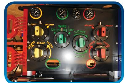
Clutched control knobs allow full control of the saw by ROV manipulation
