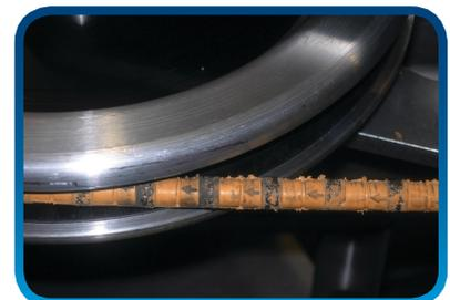
Diamond wire cutting element is easily replaced in the field, and is ideal for mixed materials and compressive cuts
