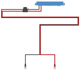
2. Install a suitably rated inline fuse or circuit breaker within the DC power cabling between the **Blue Smart IP67 Charger** and battery/batteries, located as close as practical to the battery/batteries; refer to the 'Installation > Wiring > Overcurrent protection' section for more information.
