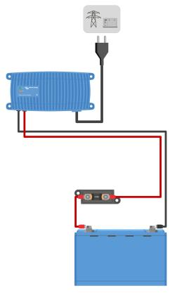
3. Connect the **Blue Smart IP67 Charger** AC power cable to a mains power outlet; after a short delay the POWER LED will illuminate and the STATUS LED will begin to blink fast.
