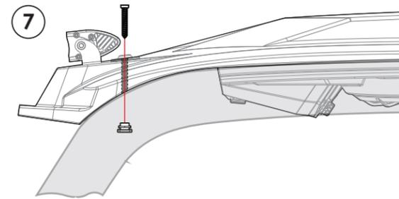
Use (2) M6 torx screws and (2) M6 flange locknuts to fasten the front of the roof. Do not overtighten the screws.
