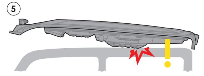
Be careful not to bump the speaker grilles while lifting the roof over the rails.
