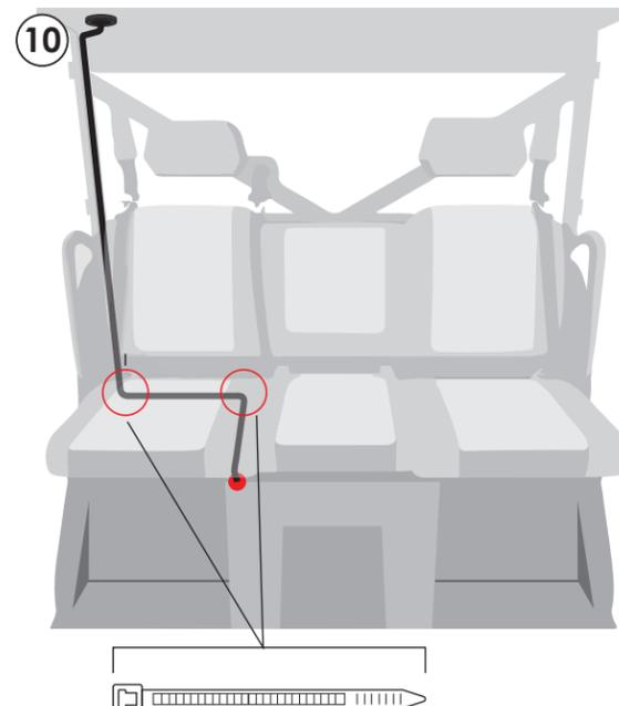
Wire the harness towards the battery and secure it to avoid it touching hot or moving parts. Extra (2) zip ties are included if needed.
