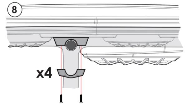
Attach the (4) center clamps with the (8) M5 screws provided to secure the roof to the center roof rail.
