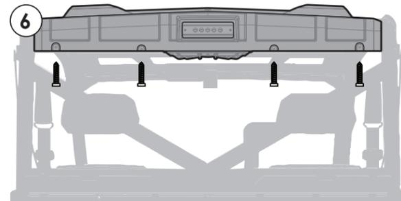
Fasten the back of the roof with the (4) M6 torx screws provided.
