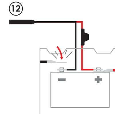
Fully reconnect the battery after the roof harness has been connected.
