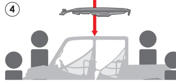
Carry the roof carefully to the vehicle and place it on the RANGER® roof rails.
