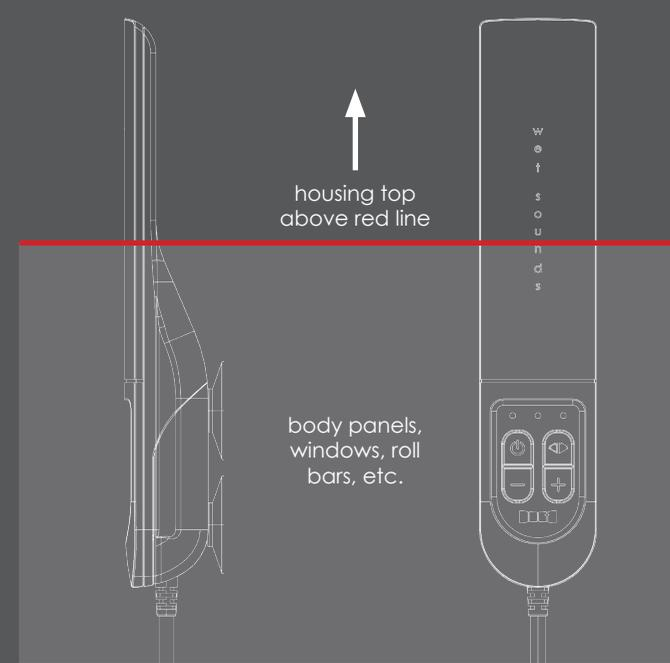
a **link plus** comes with two (2) suction cups for each unit that can be installed in the cradle for easy mounting to glass or other smooth, glossy surfaces.
