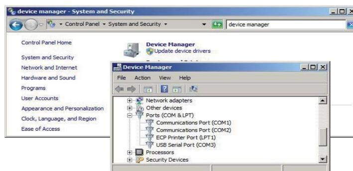
The PC sets up a virtual COM port, which later is to be used by the Service Tool.
