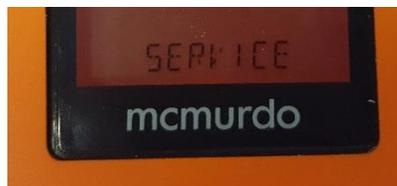
Figure 4 - Once connection between the Service Tool and the radio has been established, this will be indicated in the radio display by reading "SERVICE" as well as a soft beep from the radio.
