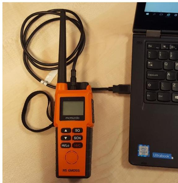
Figure 1 - Simple connection between service PC and radio.
