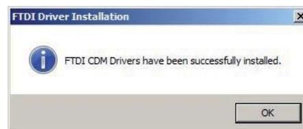
After installation, the service cable (USB end) is plugged into a free USB slot on the service PC. The PC should now be able to identify a new USB device.
