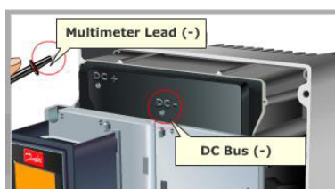
Figure 18: The multimeter should show open diode
