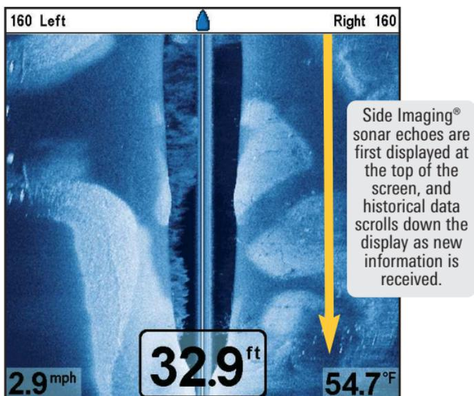
The main benefit of Side Imaging® sonar to anglers is that it provides an overall survey of a large area of water. This gives you a better understanding of the bottom topography and how structure is oriented for more efficient fishing.
