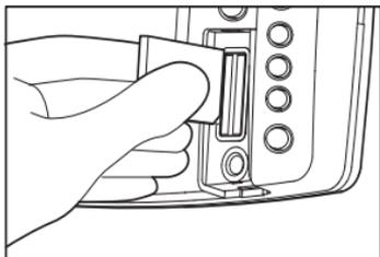
Inserting an MMC/SD
