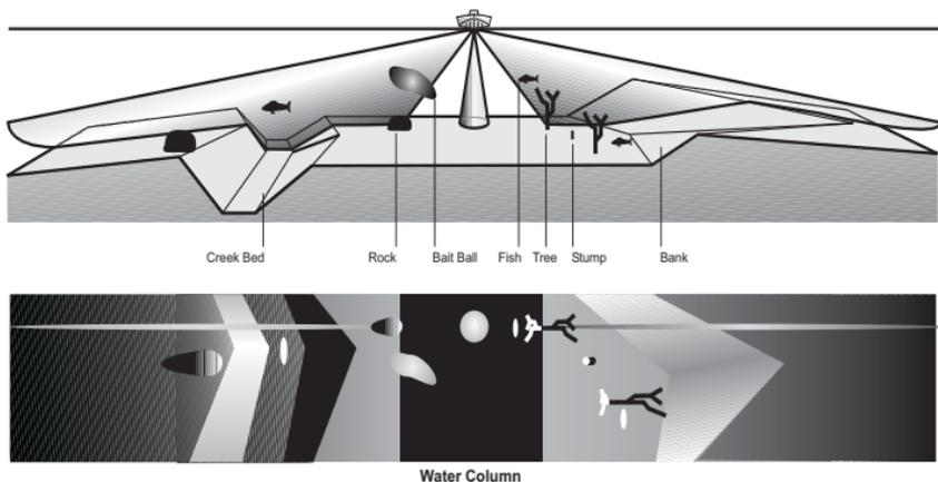
**Each time the unit pings**, a strip of data representing all the echoes received by the transducer are put together on the display to form the image that you see.
