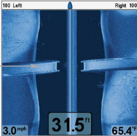
*Submerged Bridge - When there is an area directly under the boat that does not have Side Imaging® coverage, a single object may appear as two separate objects on the display.*
