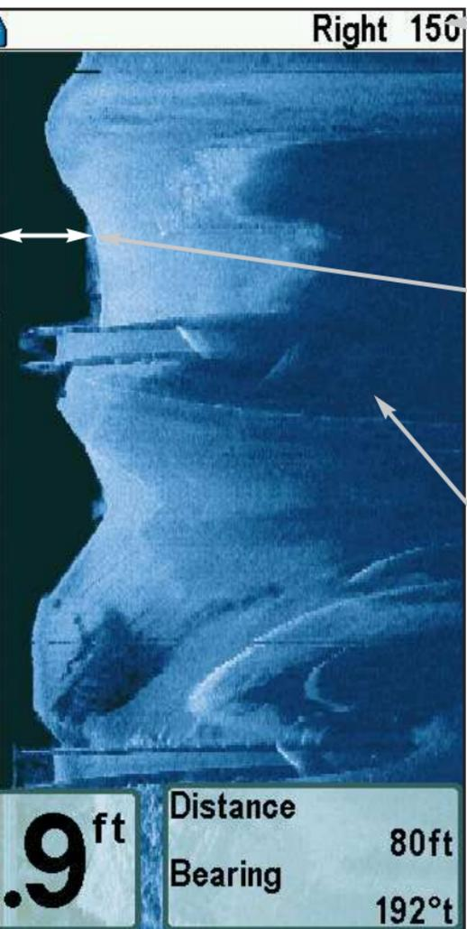
**Side Imaging® Range** - Images shown on the right side of the screen are located on the right side of your boat, and images shown on the left side of the screen are located on the left side of your boat. In this picture, the sonar is pinging 150 feet on each side.
