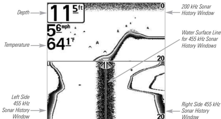
**Slanted layout:** This layout presents the two 455 kHz side sonar beams and the 200 kHz down-looking sonar beam as three panels of historical data. This layout is presented as three slanted panels. New information appears on the right and scrolls to the left.
