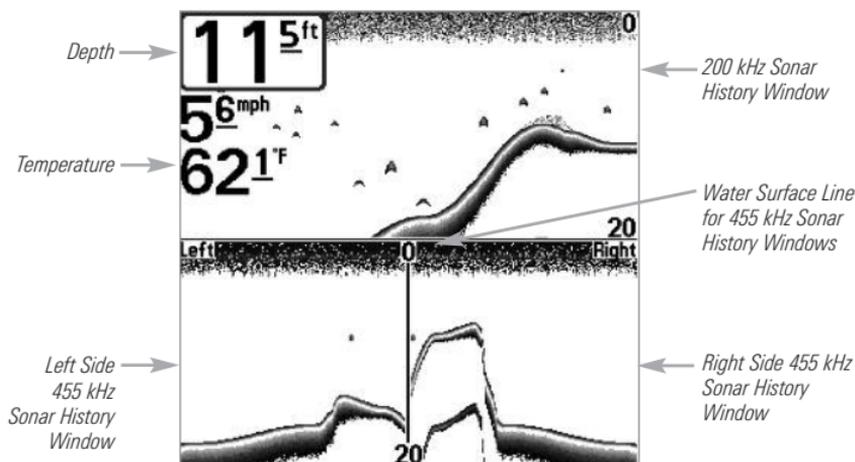
**Classic layout:** The top portion of the display presents a historical log of sonar returns from the 200 kHz down-looking sonar beam. New information in the down beam panel scrolls from right to left. The bottom portion of the display presents a historical log of sonar returns from the 455 kHz right- and left-looking sonar beams. New information appears at the top, and scrolls down the display.
