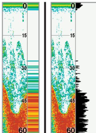
The **Wide RTS Window™** indicates the sonar intensity through the use of a bar graph. The length of the plotted return indicates whether the return is weak or strong. The depth of the sonar return is indicated by the vertical placement of the return on the display depth scale. The Wide RTS Window™ does not use grayscale.
