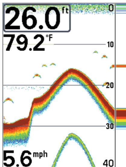
**Structure ID**<sup>®</sup> represents weak returns in blue and strong returns in red when Sonar Colors is set to Original. If the Sonar Colors palette is changed, the Structure ID<sup>®</sup> will display the strongest return as specified by the palette. See *Sonar Menu Tab: Sonar Colors* for more information.
