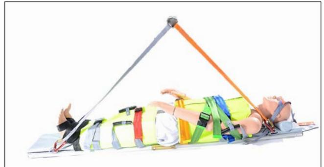
Figure 20 - Using Four Point Lifting Bridle
