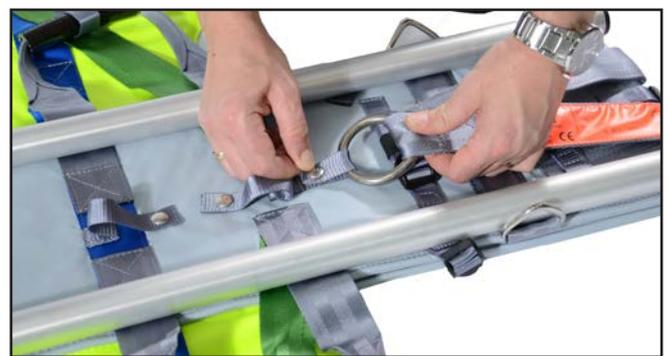
Figure 7 - Release vertical lifting rings
