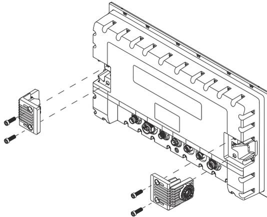
5. Mount the unit to the bracket using the knobs. Hand tighten only. The ratchet teeth in the bracket and unit case ensure a positive grip and prevent the unit from changing from the desired angle.
