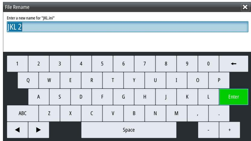
You remove the virtual keyboard without entering information by pressing the **Exit** key.
