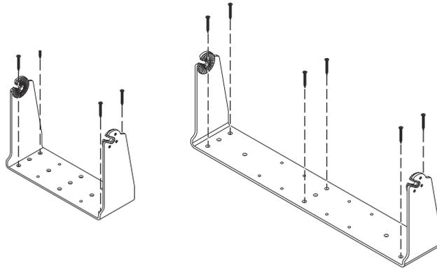
4. (16" units only) Using the screws provided in the gimbal kit, fasten the gimbals to the unit.
