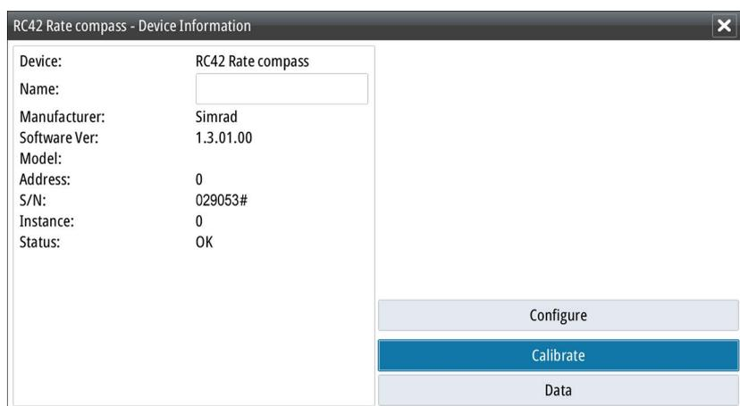
All devices allow allocation of an instance number in the configure option. Set unique instance numbers on any identical devices on the network to allow for the unit to distinguish between them. The data option shows all data being output by the device. Some devices will show additional options specific to the device.
