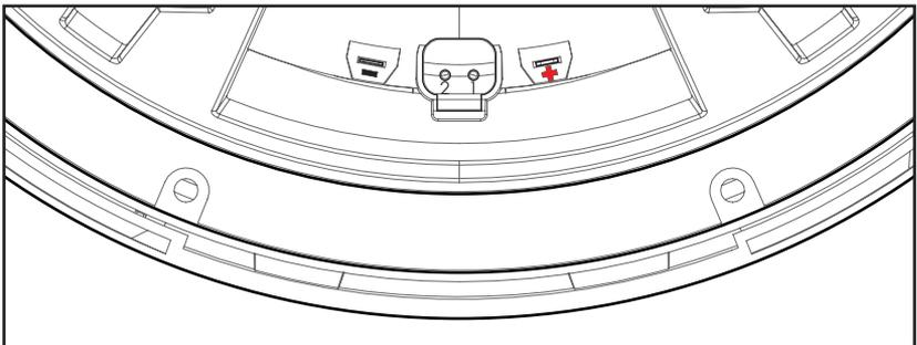
**Note:** ZERO Series has a standard Deutsch connector compatible connection. (PN: DT04-2P) PIN 1 (+) PIN 2 (-)
