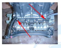
5.5 (Below) Remove the remaining starter bolt with a 12mm socket.
