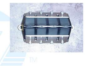
2.10 (Below) Look at each petal-to-cage surface and check for gap. If a gap of more than 0.015" is present, replace the petals.
