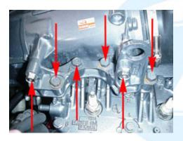
3.3 (Below) Remove the thermo sensor from the exhaust pipe by removing the two 10mm bolts.
