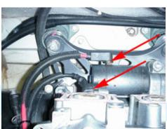
4.3 (Above) Remove the starter lead nut & washer with a 10mm socket and block ground bolt with a 12mm socket.
