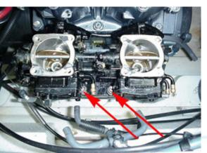
2.6 (Left, Below) Remove the 4 carb base mounting bolts with a 12mm wrench and remove the carb assembly from the hull.
