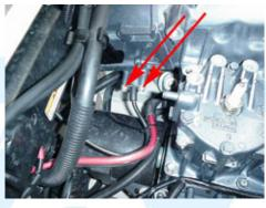
3.4 (Below) Loosen the clamp around the waterbox coupler and slide the waterbox back, out of the boot.
