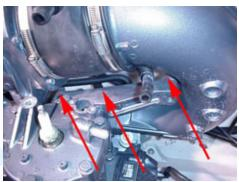
3.5 (Above) Remove the three 12mm bolts from the pipe brace and remove the brace from the hull.
