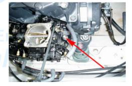
2.5 (Right) Loosen the gas tank cap to relieve pressure. Be sure the fuel switch is turned to the "OFF" position, and be aware of any fuel that may spill from the hoses. Make sure the hull is clear of any gasoline fumes before continuing work, especially with power tools. Disconnect the pulse lines, fuel in & fuel return lines from both carbs. Mark each line so you can replace them later to the correct position.
