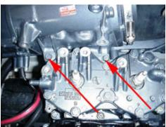
3.2 (Above) Remove the two 12mm bolts securing the exhaust pipe to the cylinders.
