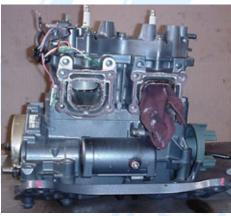
5.3 (Above, Right) Stuff a rag into an open exhaust port. This will prevent the engine from turning over while removing the flywheel and PTO coupler. Remove the flywheel nut with a 17mm socket. Use a universal flywheel puller to remove the flywheel from the shaft. Do not ship the flywheel key to SBT. Pull the starter gears out of the housing.
