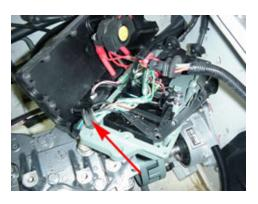
4.6 (Below) Remove the four 12mm engine mount bolts. Note the number and position of all engine mount shims.
