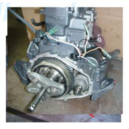
5.4 (Below) Remove the pulse lines from the case.
