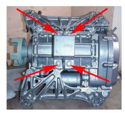
5.2 (Below, Right) Remove the 7 10mm bolts from the flywheel housing and remove the cover. If the cover grommet stays with the gasket, bend it free and remove the old gasket.
