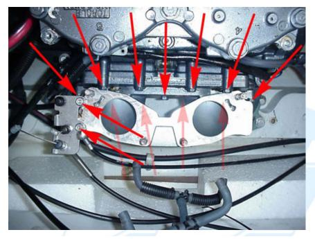
2.7 (Above) Use a 10mm socket to remove the two bolts securing the cable bracket, then remove the 11 10mm bolts from the intake manifold. Remove the manifold from the hull.
