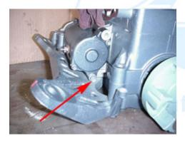
5.6 (Below) Use a chain wrench to unscrew the PTO coupler. After it spins free, remove the rag from the exhaust port.
