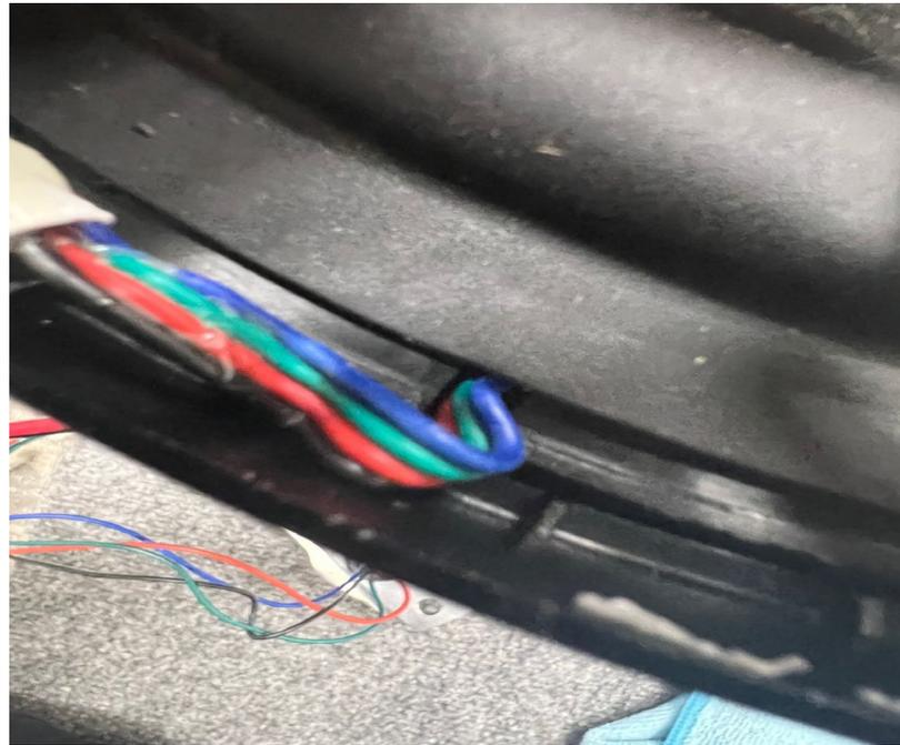
The RGB wire sits in a notch in the housing that lines up with the notch on the mid bass. Once you line them up your led wire will pass through.
