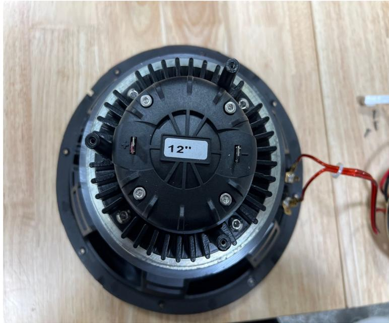
Once the Cross over is removed you then will see the HLCD that houses the Diaphragm. There are (4) 3mm Allen screws that hold the cover on.
