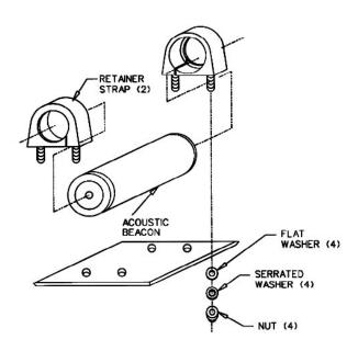
Figure 7. Method of Installing the N30A21A Mounting Kit
