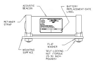
Figure 8. Securing Beacon in N30A21A Mounting Kit
