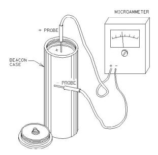
Figure 22. Beacon Off-Current Test Set-Up
