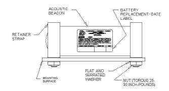
Figure 14. Securing Beacon In N30A21A Mounting Kit
