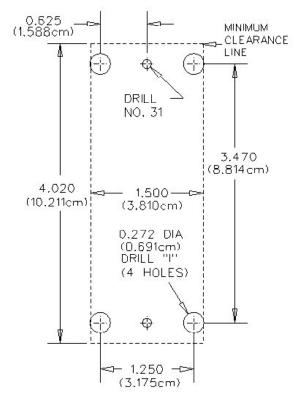
NOTE: ADDITIONAL CLEARANCE IS DESIRABLE AT SWITCH END OF BEACON
