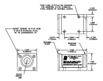
Figure 9. N30A29 Mounting Kit Installation Details
