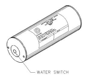
Figure 2. Water Switch Location on Beacon
