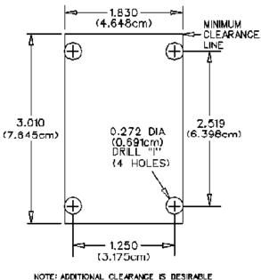
NOTE: ADDITIONAL CLEARANCE IS DESIRABLE AT SWITCH END OF BEACON
