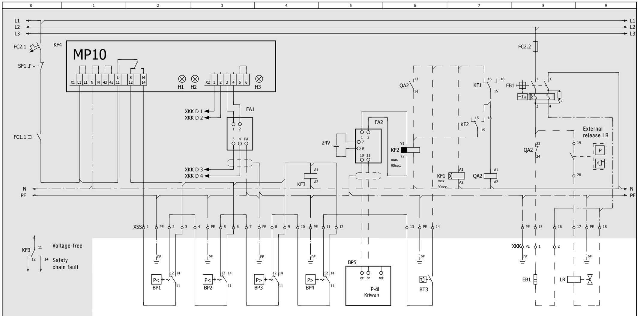
The circuit diagram is a system scheme for assignment and order of the safety chain, without error messages and installation arrangement (whether inside or outside the Ex zone).
