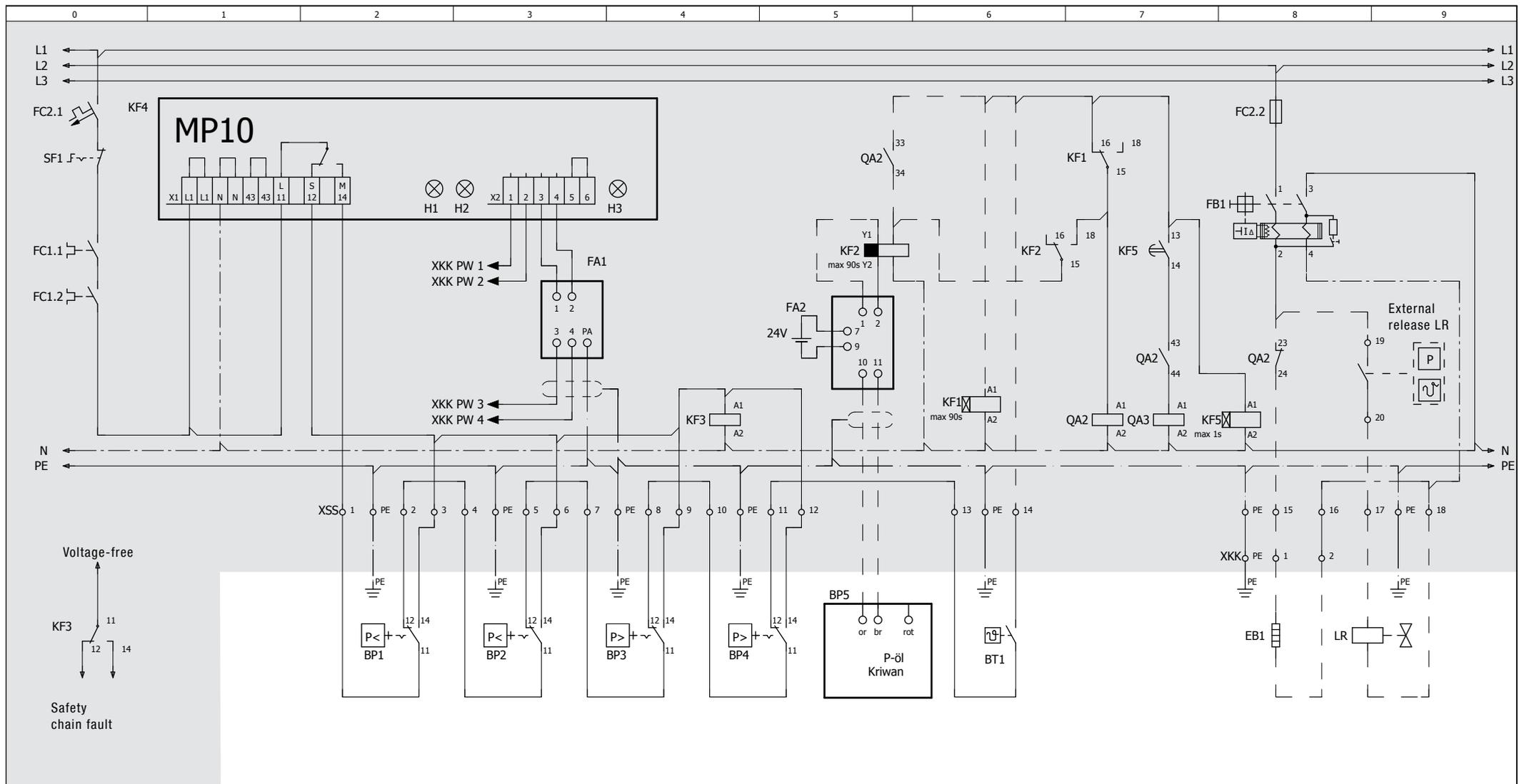
The circuit diagram is a system scheme for assignment and order of the safety chain, without error messages and installation arrangement (whether inside or outside the Ex zone).
