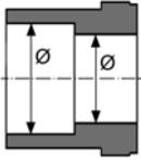
Fig.18: graduated internal diameter
