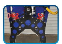
Multiple ROV compliant handles for vertical or horizontal deployment
