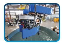
Low profile syntactic flotation package is rated for 3000msw (9843fsw)
