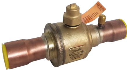
Danfoss shut-off ball valves, type GBC (90 bar), GBCT (140 bar) are manually operated shut-off valves for CO<sub>2</sub> refrigeration systems, in order to open and to shut off inner flow path by operating the valve spindle.
