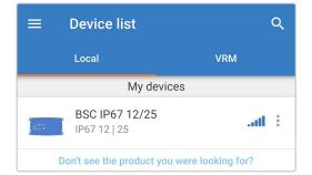
4. Select the **Device options** icon (three vertical dots on the right side of the description) to access the dropdown menu.
