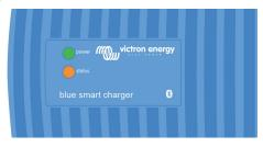
Using a Bluetooth enabled device (mobile phone or tablet), open the VictronConnect app and locate the Blue Smart IP67 Charger in the Device list Local page, then connect to the device (the default PIN code is stated on a label located on the back of the charger, or try 000000 if there is no label).
