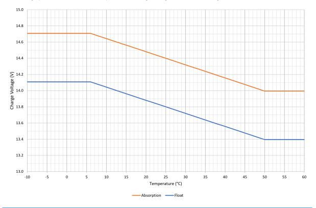
Refer to the graph below for the default temperature vs charge voltage curve for 12V chargers:
