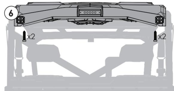
Fasten the back of the roof with the (4) M8 torx screws provided.
