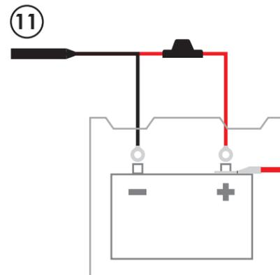
Connect the red wire to the positive battery terminal. Followed by the black wire to the negative terminal.
