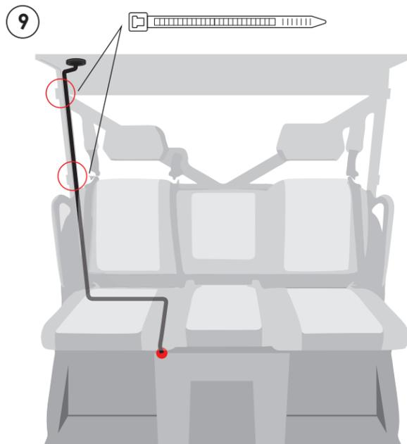
Secure the wiring harness to the post by using (2) zip ties near the locations marked above.
