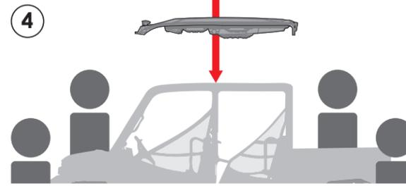
Carry the roof carefully to the vehicle and place it on the DEFENDER roof rails.
