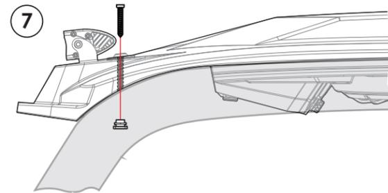
Use (3) M6 torx screws and (3) M6 flange locknuts to fasten the front of the roof. Do not overtighten the screws.
