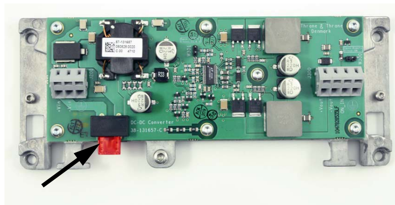
Figure 4-1: Fuse in the SAILOR 6090 Power Converter
