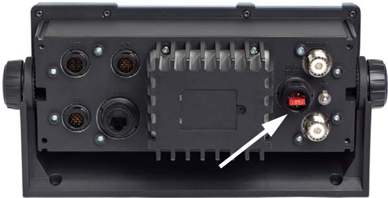
Figure 4-1: Fuse in the power connector
