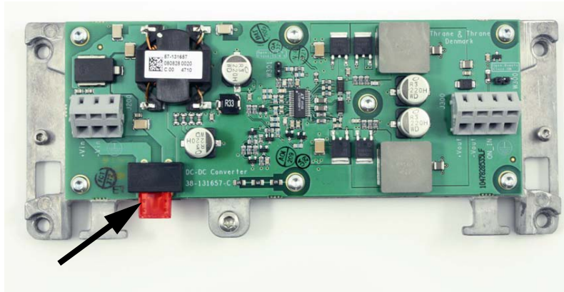
Figure 4-2: Fuse in the SAILOR 6090 Power Converter
