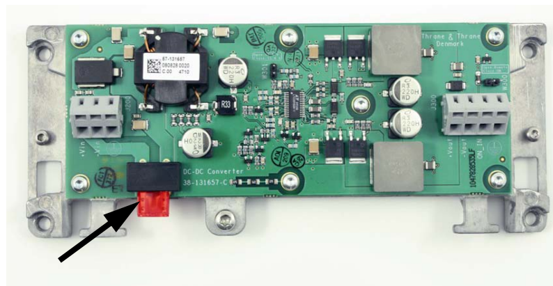
Figure 4-1: Fuse in the SAILOR 6090 Power Converter
