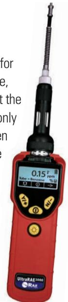
To begin measuring, turn on the UltraRAE 3000. This screen is shown, which includes the CF (correction factor) and measurement gas type (benzene, butadiene, etc.) for calibration reference:
