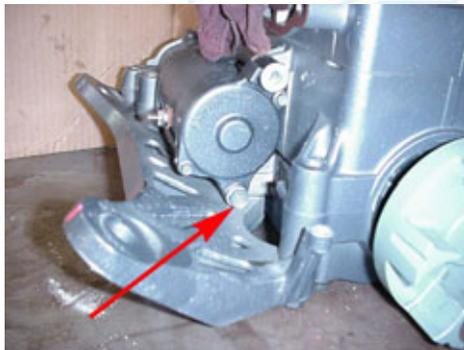
5.6 (Below) Use a chain wrench to unscrew the PTO coupler. After it spins free, remove the rag from the exhaust port.
