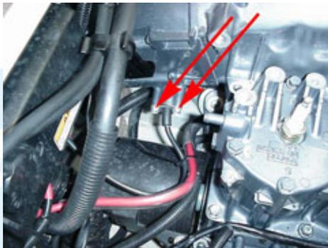
3.4 (Below) Loosen the clamp around the waterbox coupler and slide the waterbox back, out of the boot.
