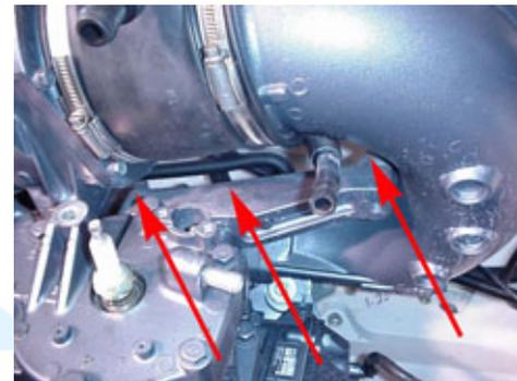
3.5 (Above) Remove the three 12mm bolts from the pipe brace and remove the brace from the hull.
