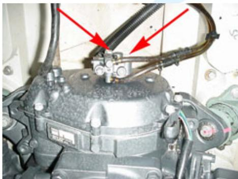
4.2 (Below) Remove the grease line from the flywheel housing.
