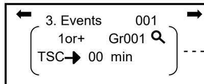
Note that the 301C controller/E<sup>3</sup>Point system reports time since calibration in days. Therefore, setting the time limit to 5 minutes would cause an event to activate 1140 minutes (1 day) after calibration.
