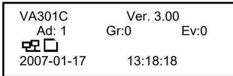
If one or more of the connected devices is in an alarm mode, the controller will only scroll between the main information screen and the screens for device(s) in alarm mode. In this case, you must scroll manually to view screens for other devices.
